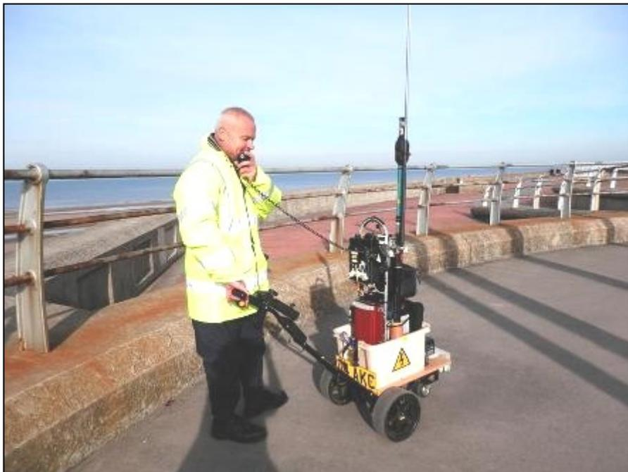
Dave G4AKC, operating from the promenade at Blackpool; even with the tide out Dave is still in the Fresnel Zone due to the wet sand. In his experiments he has found a very slight drop in performance as the tide goes out. Notice no connection between the trolley and the ground other than the insulated wheels.
