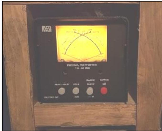
A fairly recent addition to the ever increasing number of black boxes, the Palstar PM2000 Wattmeter. Not the cheapest meter available by far but what it has over the others is that it can display a True Active Peak Power reading. This is important when measuring power output when on SSB, especially when using high power amplifiers.
